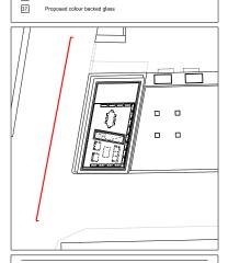
Proposed mechanically operable roof light (to form balustrade when in open position)
