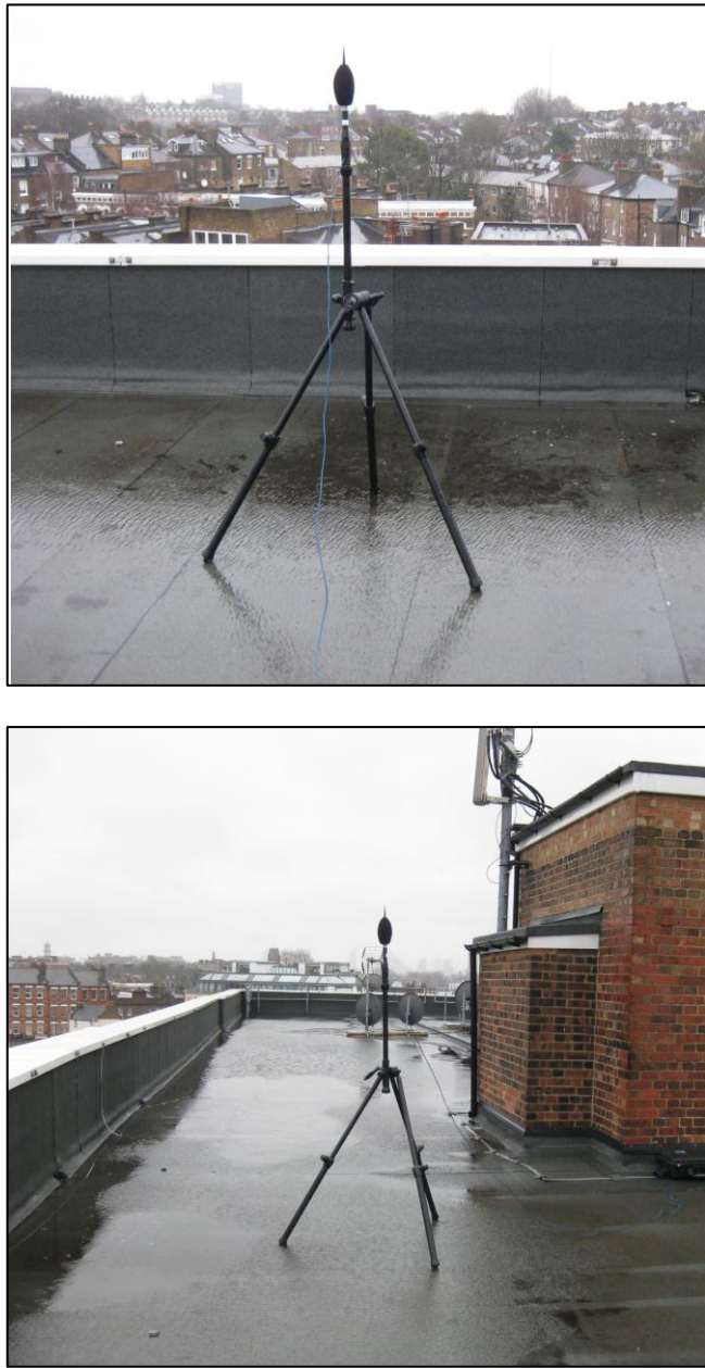
Figure 3: Photos of Noise Survey
