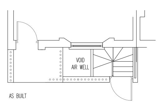
THERE IS NO CHANGE TO THE RAILING FRONTING ONTO CHALCOT ROAD. THE RAILING THAT IS PERPENDICULAR HAS BEEN MOVED APPROXIMATELY 500 mm TO THE RIGHT
