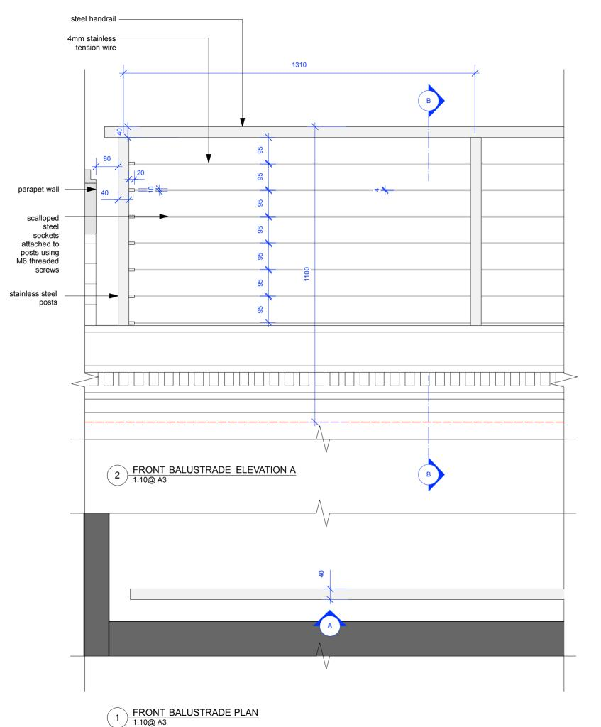
steel handrail 4mm stainless tension wire threaded in to scalloped steel sockets attached to posts using M6 threaded screws stainless steel posts plate securely fixed in to parapet wall & made watertight red line indicates finished floor level FRONT BALUSTRADE SECTION BB
