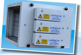
produce UV light at 254nm, the most efficient UV-C wave length, which converts the ozone to hydroxyl free radicals. Purified Air's UV-C odour control system also features a photo catalytic liner, which enhances the production of hydroxyl free radicals when exposed to UV light. Free radicals are natural air cleansing agents and are strong oxidants. They are significantly more powerful than plain ozone.
