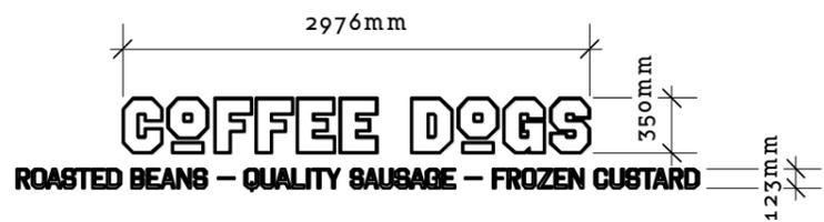
REVERSED OUT, BUILT UP TO A DEPTH OF 50MM, ARCHITECTURAL LETTERING IN 3MM ALUMINIUM WITH FIXING BACK TO SIGN RAIL. DETAIL TO BE SUPPLIED BY SIGNAGE CONTRACTOR
