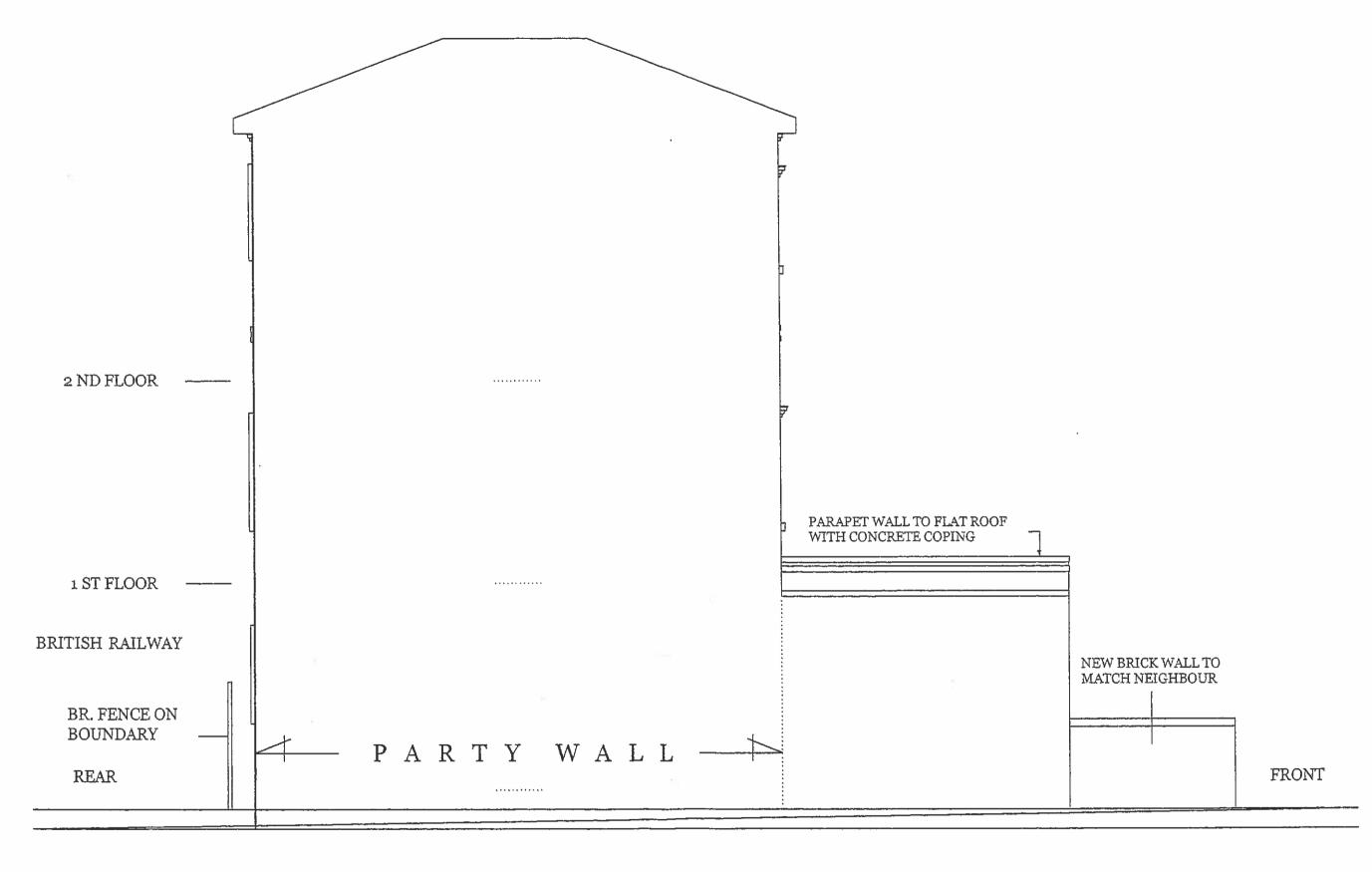
PROPOSED SIDE ELEVATION 1:50 221A BELSIZE ROAD LONDON NW6 4AA
