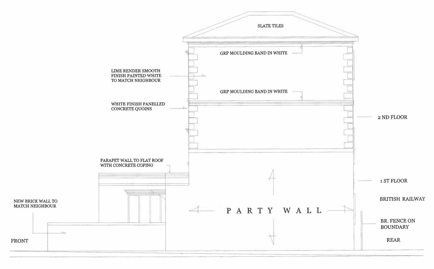
PROPOSED SIDE ELEVATION 1:50 221A BELSIZE ROAD LONDON NW6 4AA
