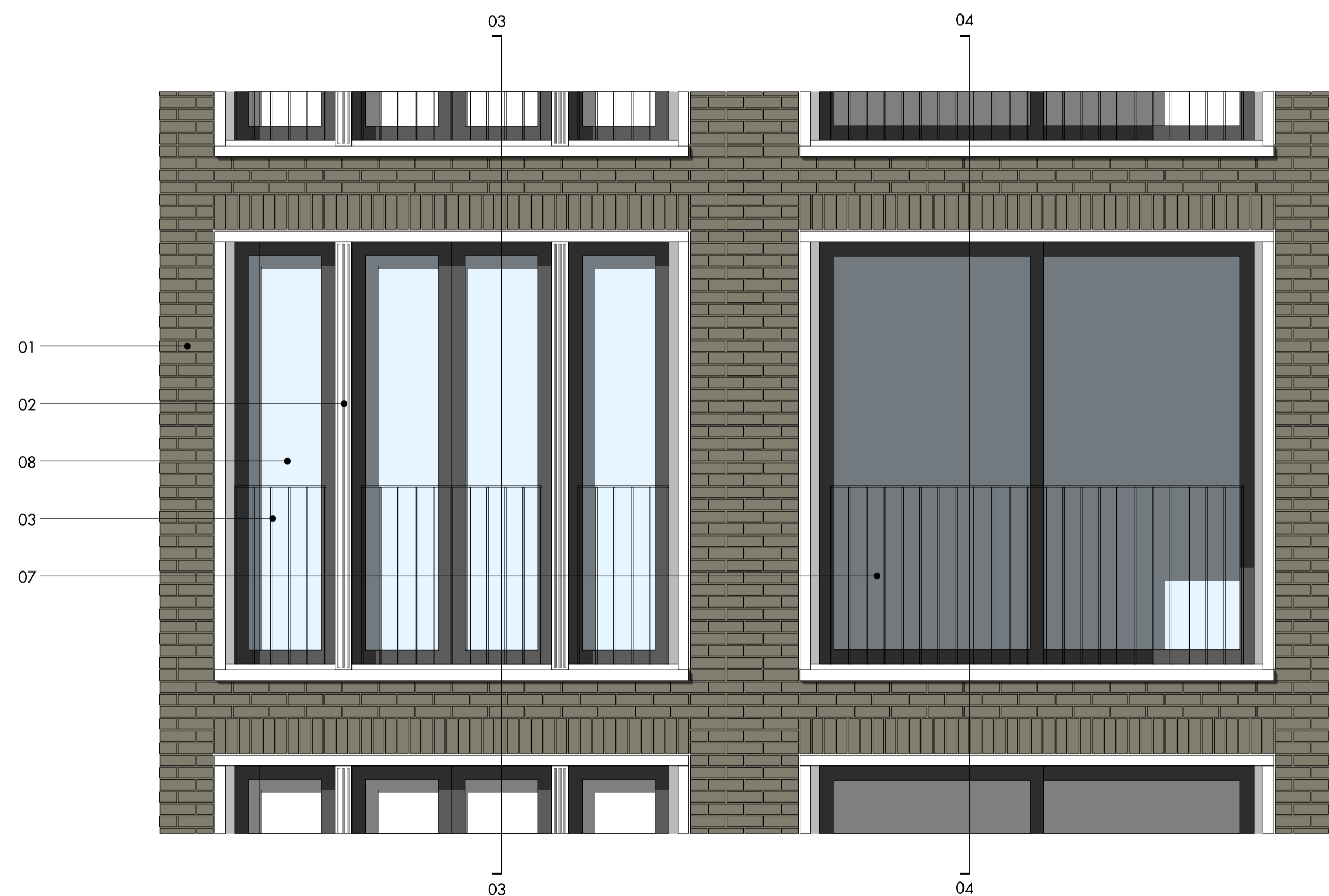
02 TYPICAL WINDOW & BALCONY ELEVATION
