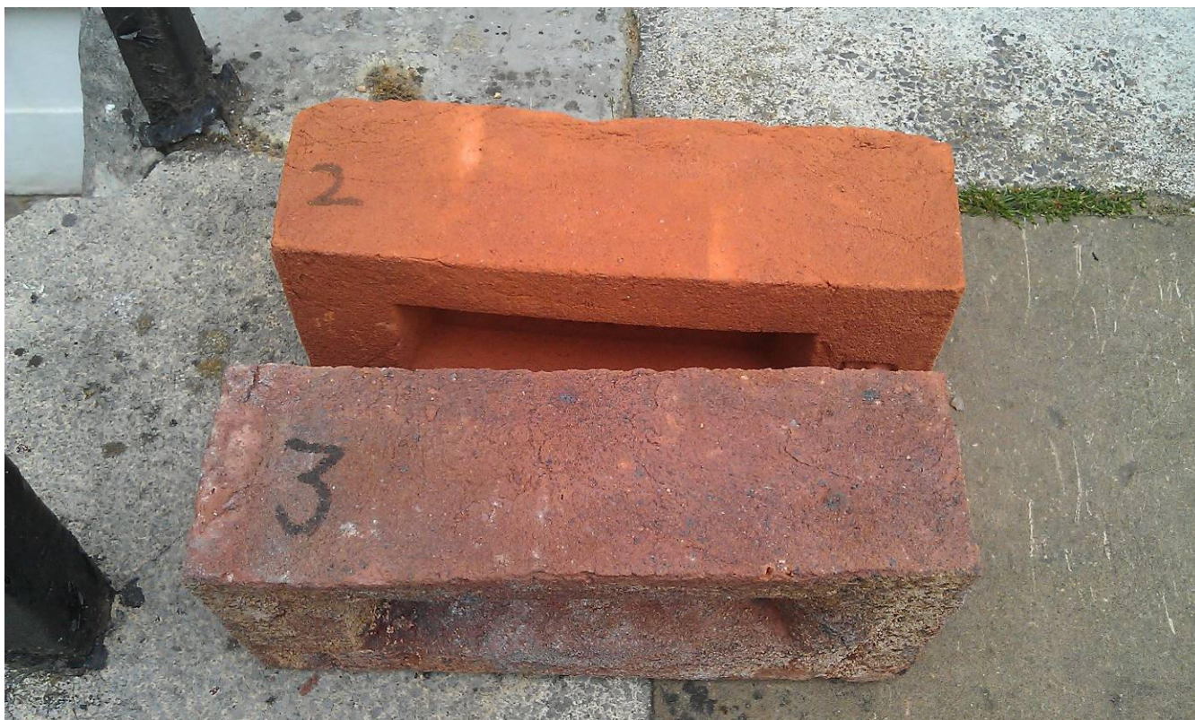
Photo 4: View of Lambs bricks specified in the repair to the external wall:
