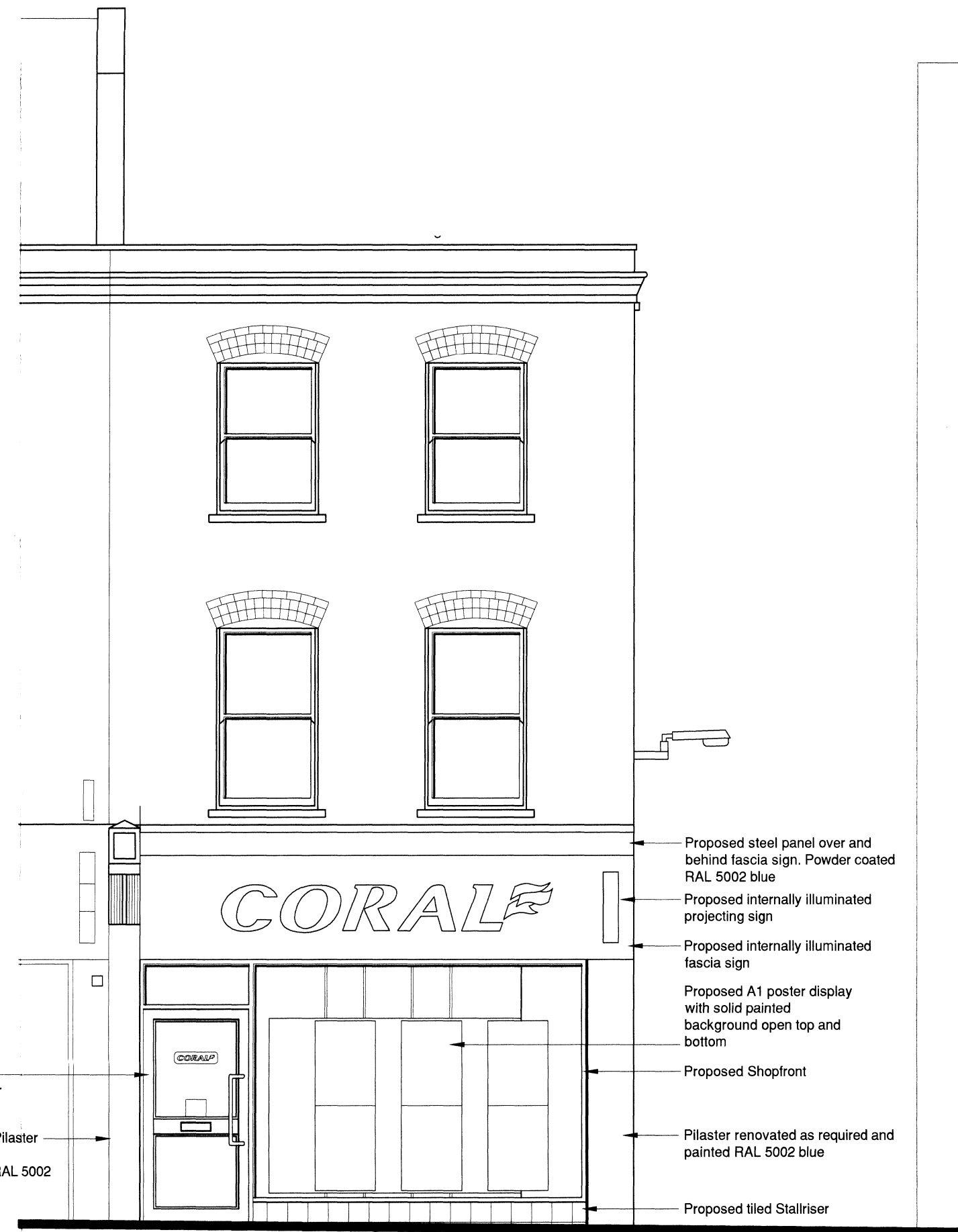
PROPOSED SHOPFRONT ELEVATION (NORTH EAST)
