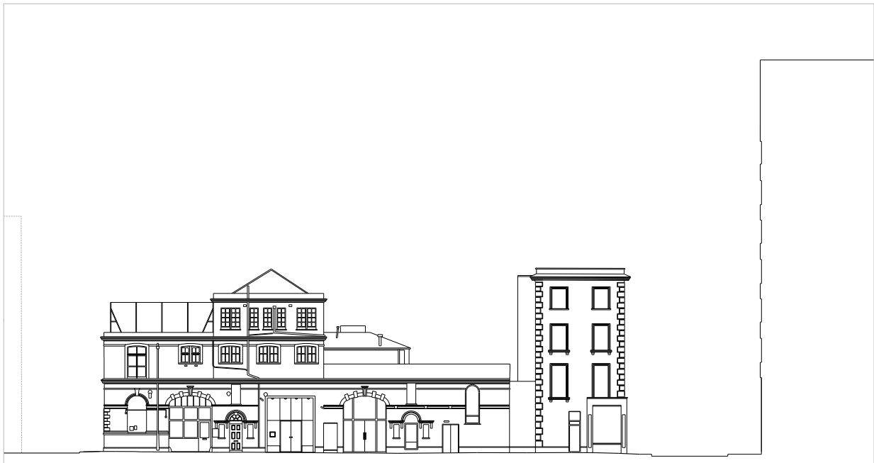
Fig. 5.3: Existing south New Oxford Street elevation. Where windows need to be restored, they would be replaced with identical windows, but doubleglazed to adhere to ecological standards.
