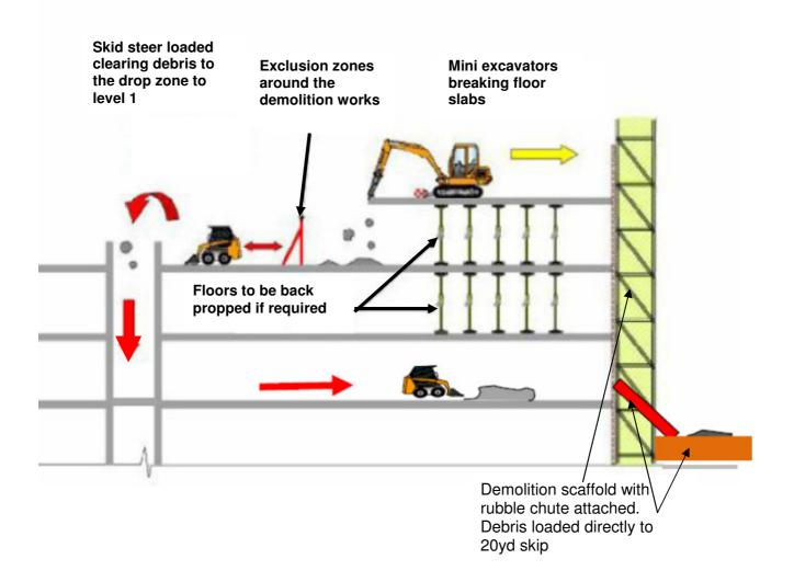
The drop zone on level 1 will have a full exclusion zone erected and signage this area will be strictly controlled by the Project Manager and the Demolition Supervisor whilst in operation by radios.
