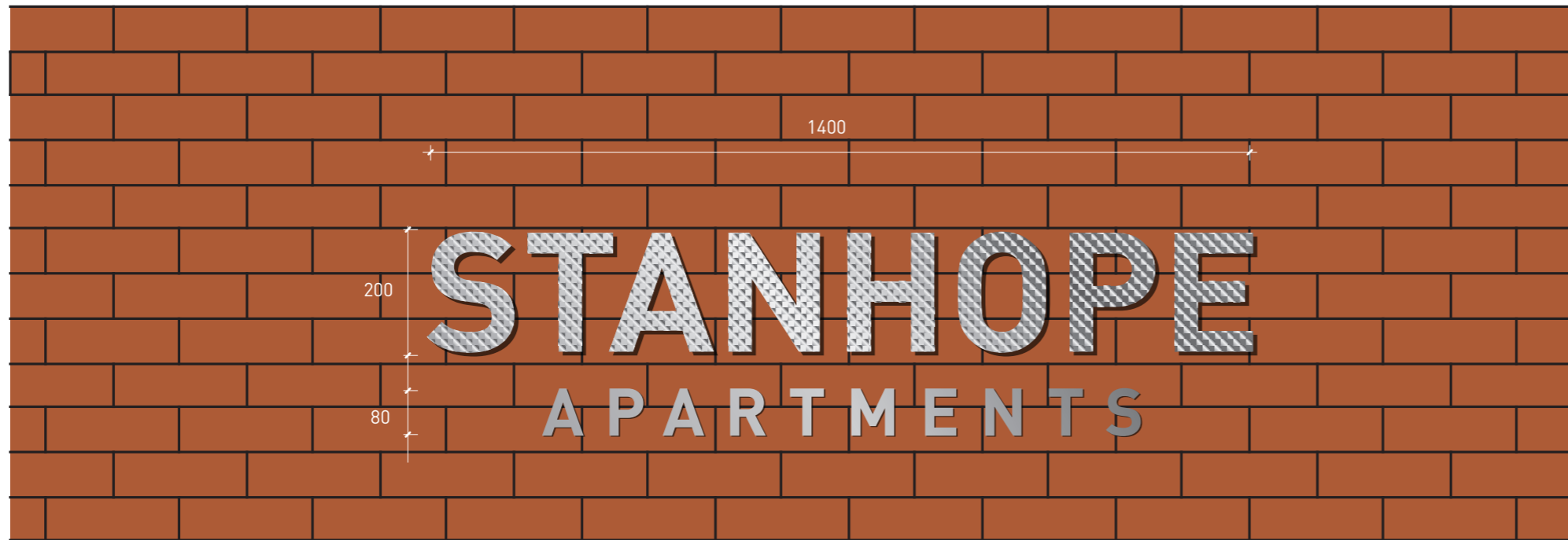
Elevation of Entrance Sign Scale 1:10 @ A3
