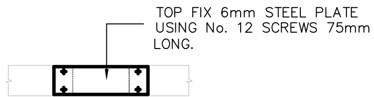
PLAN ON NOTCH REPAIR
