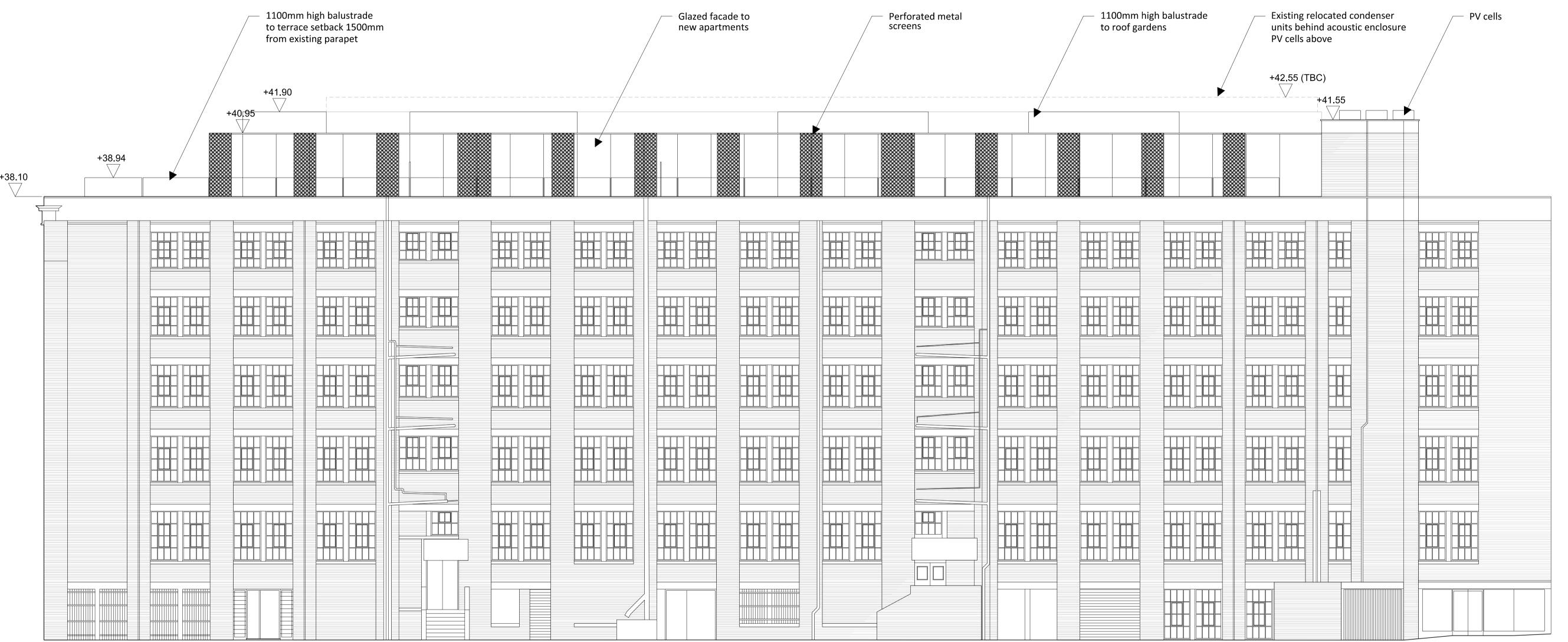
West elevation as proposed 152\_312 Scale 1:100 @ A1
