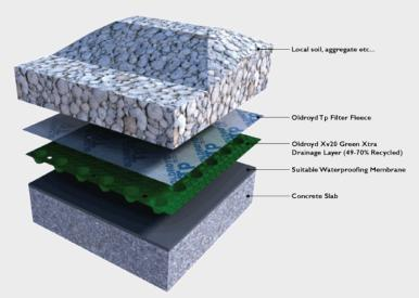
The layer build-up for brown roofs is similar to that employed for flat green roofs - the key difference being the fact that the top layer consists of a varied range of growing mediums, usually collected from the local area. These growing mediums are usually selected to maximise biodiversity. The diagram on the left shows a typical example.
