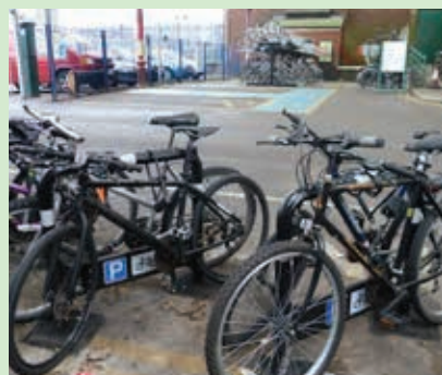
The RidgeRacks design incorporates a ridged top to reduce lock movement
