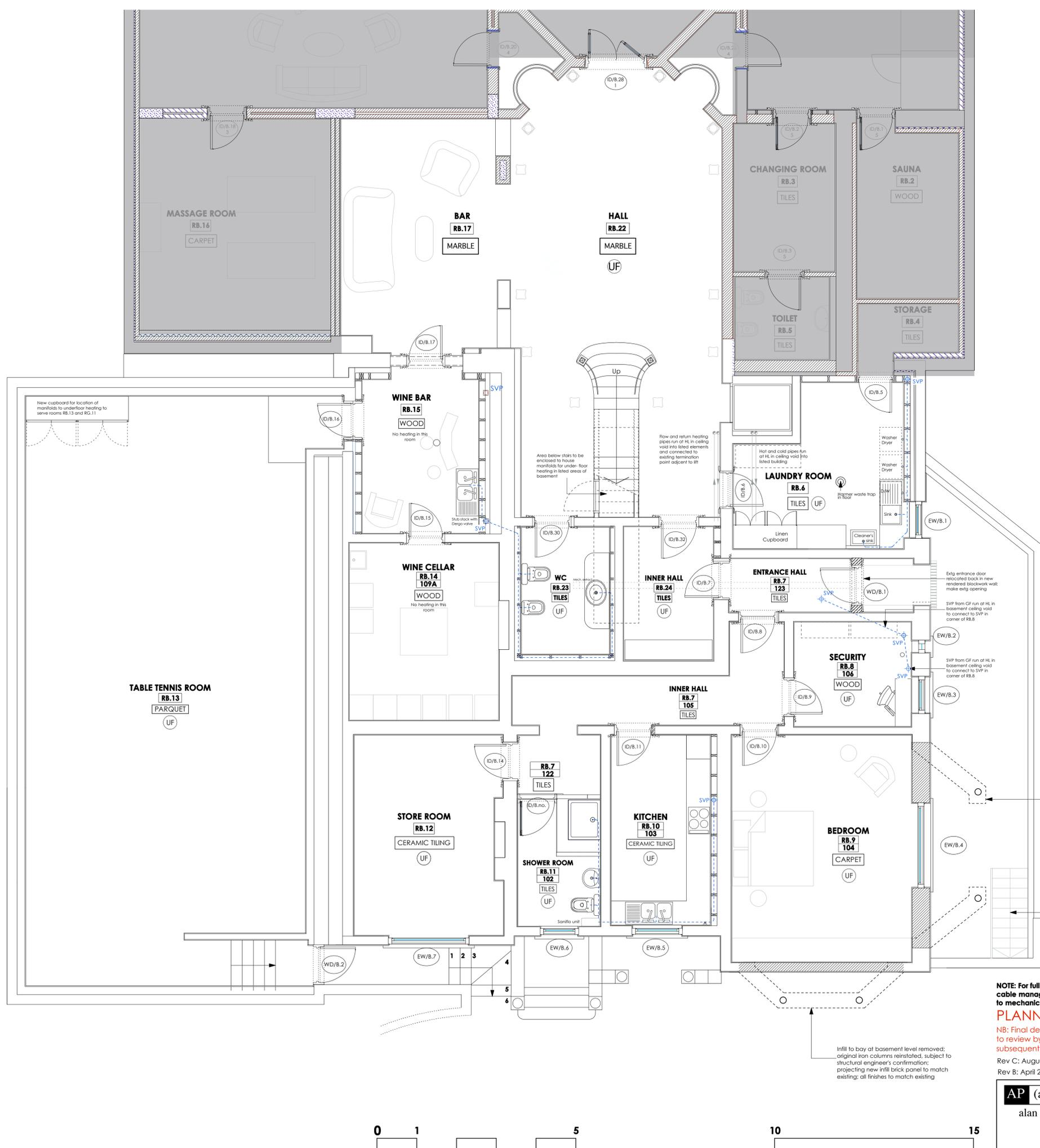
Infill to bay at basement level removed; original iron columns reinstated, subject to structural engineer's confirmation; existing HW window and projecting sill moved back to main wall line; all finishes to match existing
