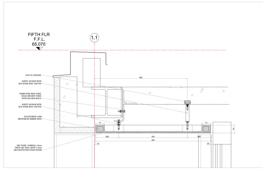
TYPICAL SECTION (BETWEEN GRIDLINES - SOUTH ELEVATION)
