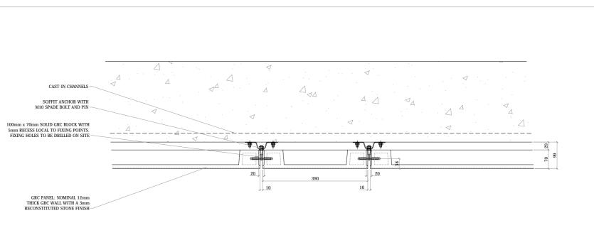
TYPICAL SECTION (ACROSS PANEL JOINTS - NORTH, WEST & EAST ELEVATIONS)
