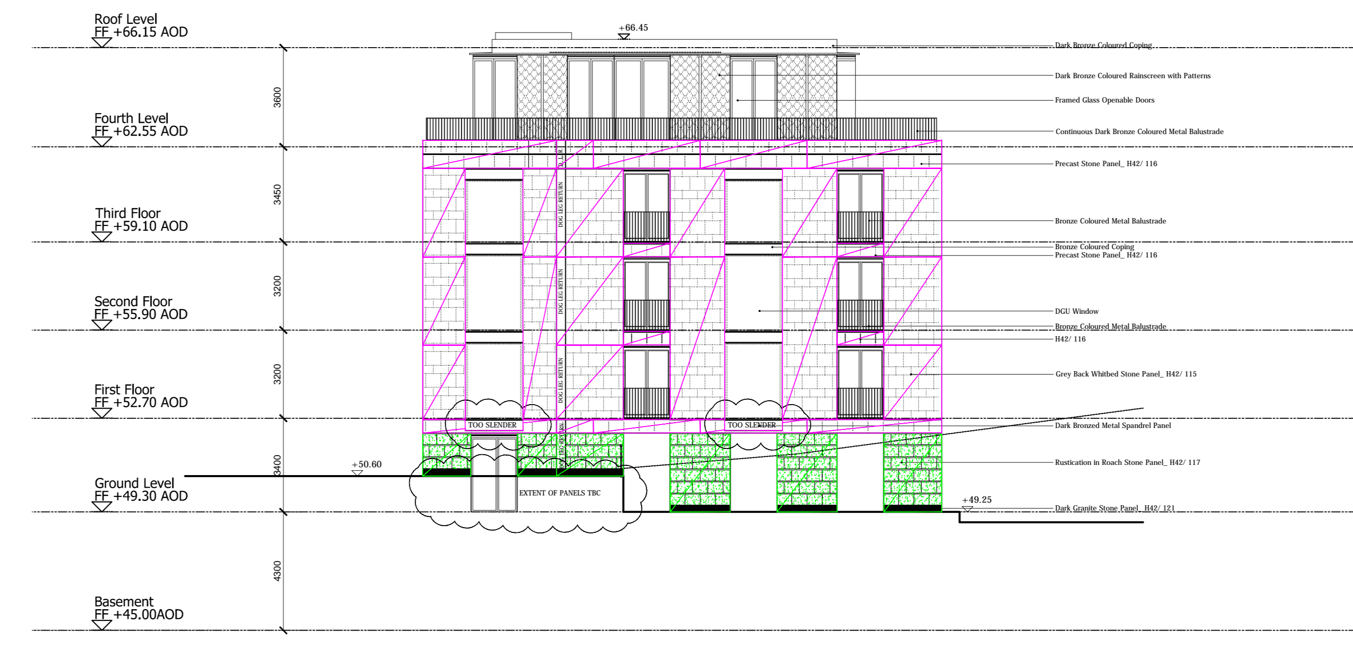
BLOCK 3 - North Elevation
