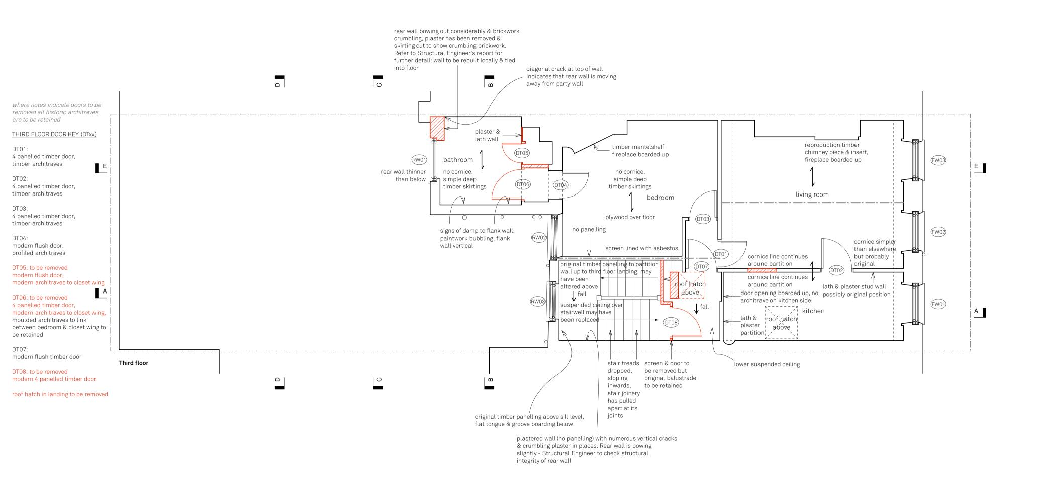
ALL PANELLING, INCLUDING PANELLING EXPOSED DURING CONSTRUCTION WORKS, TO BE RETAINED & REPAIRED.
