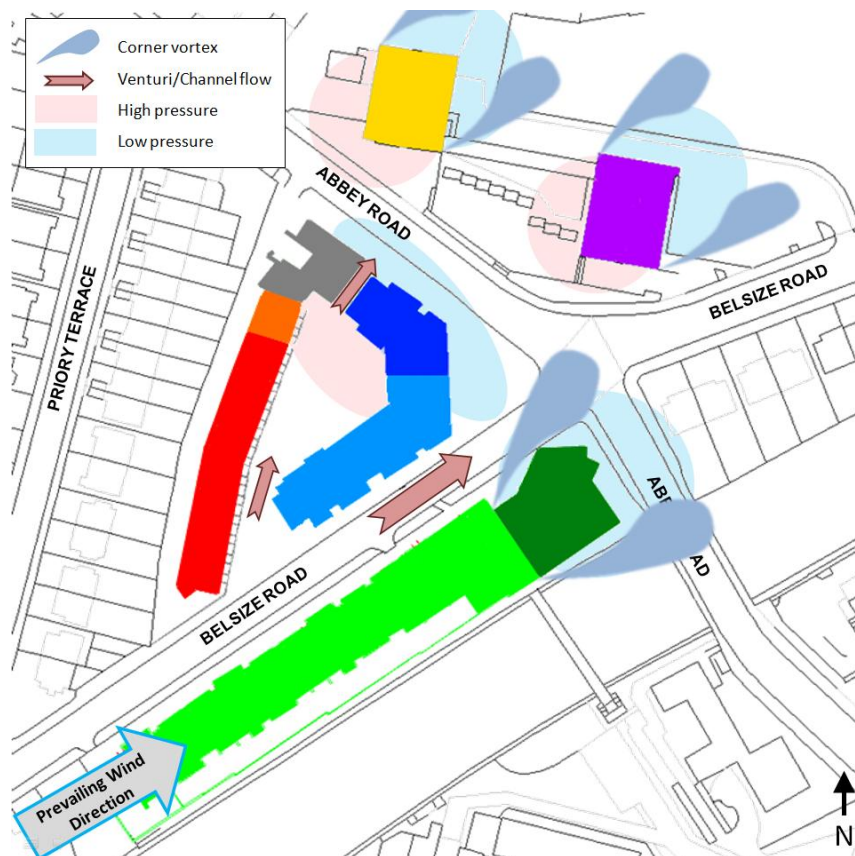
Figure 5.2 Schematic of expected flow structure from prevailing winds (from the South West) at the Abbey road regeneration site.
