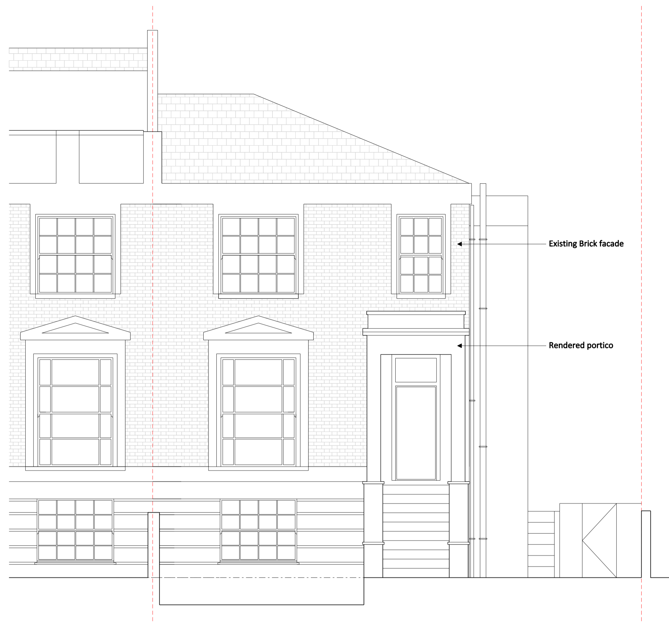
1 Front Elevation as Existing 193_031 Scale 1:50 @ A1
