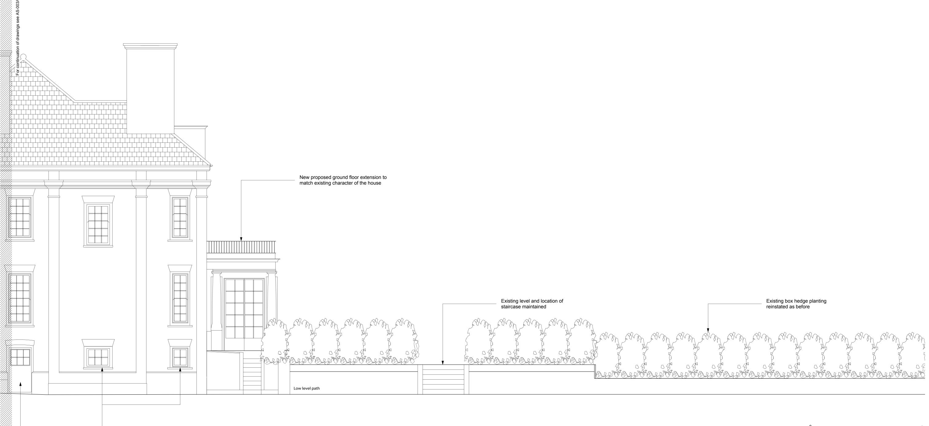
Existing door to the basement to be retained New proposed windows to match existing
