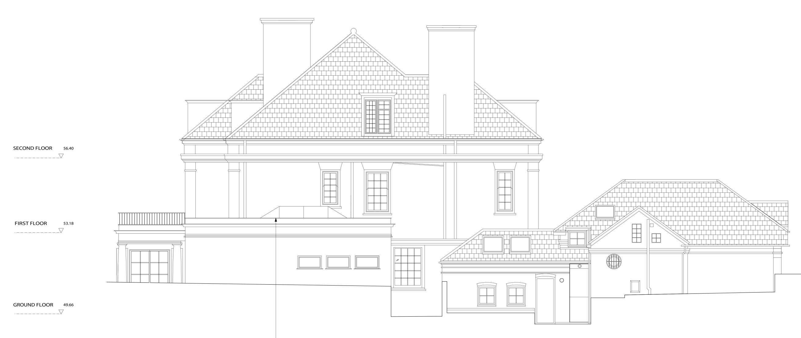
New proposed raised flat roof with traditional rooflight
