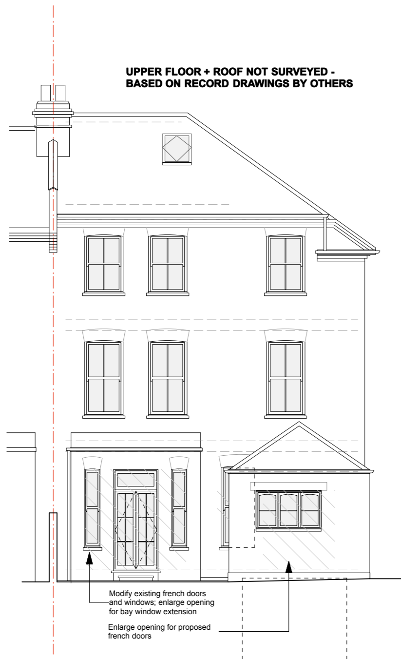
Rear Elevation : Existing Scale 1:100
