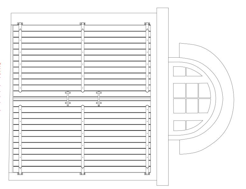
Painted timber external outward opening framed & braced door.
