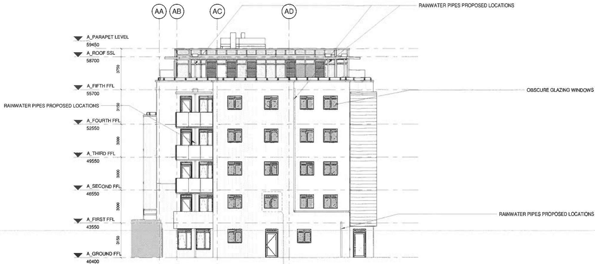
A - North West Elevation 1 : 100
