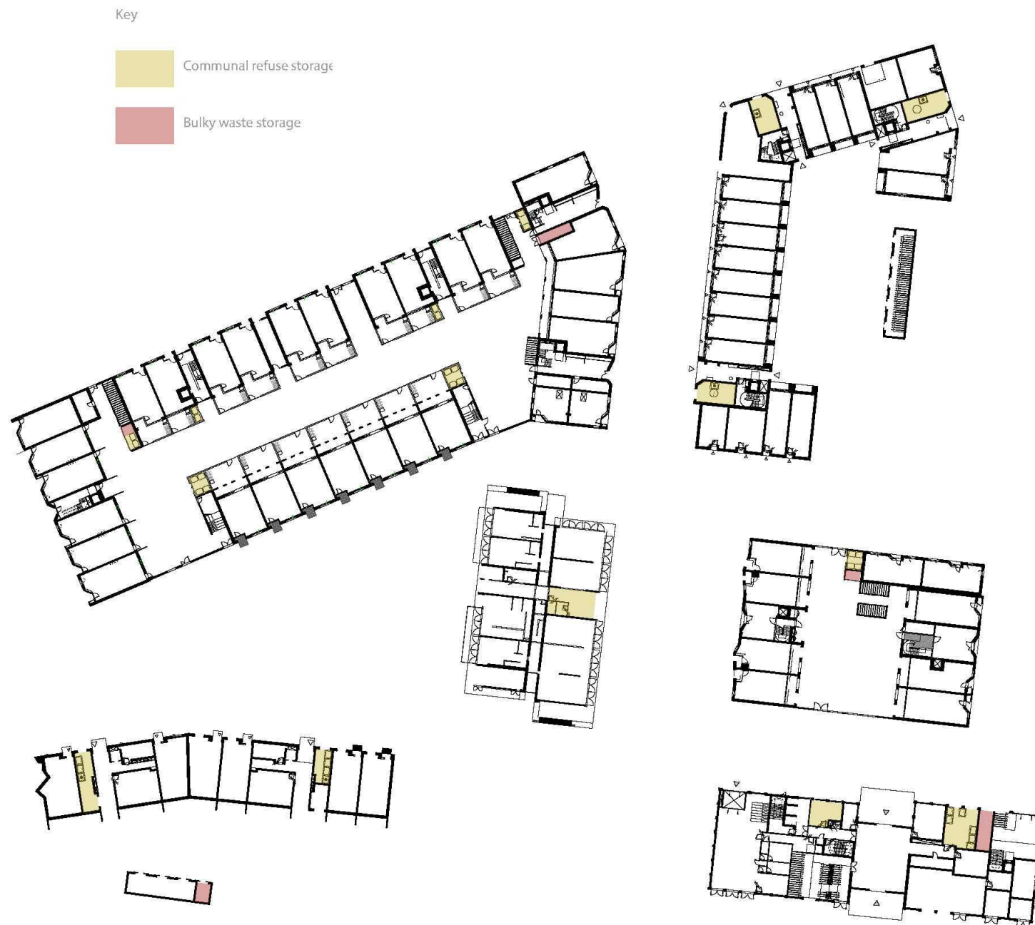
Figure 8.1: Waste Storage Areas
