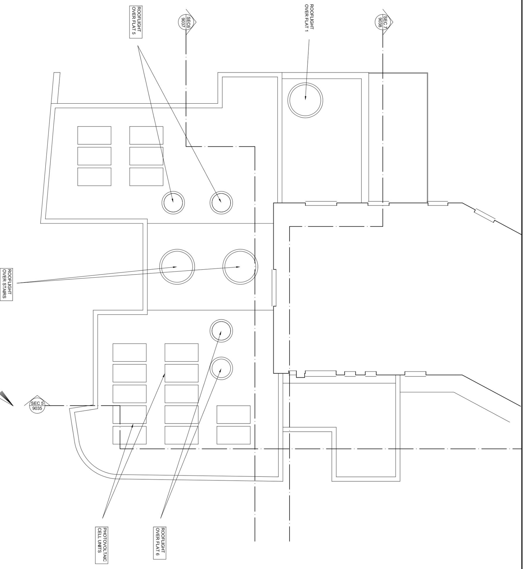
P02 - REVISED & UPGRADED TO INCLUDE PANASONIC HIT PHOTOVOLTAIC MODULES - x 18 ROOF PARAPET RAISED NOM 400mm TO OBSCURE PV UNITS FROM VIEW. 06.12.13
