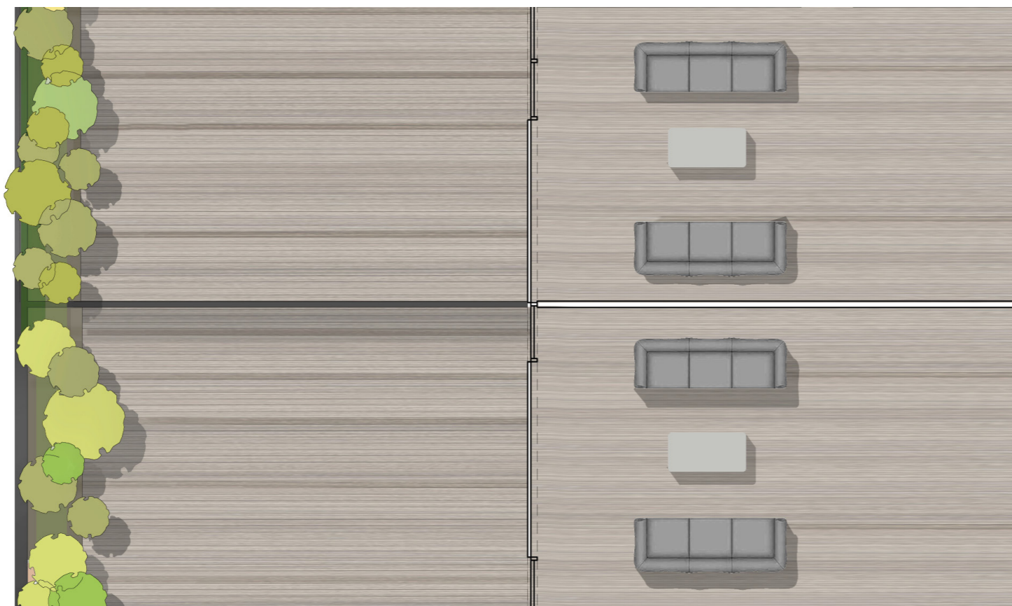
Plan of fourth floor terrace to residential units with timber decking and integrated planting boxes [not to scale]
