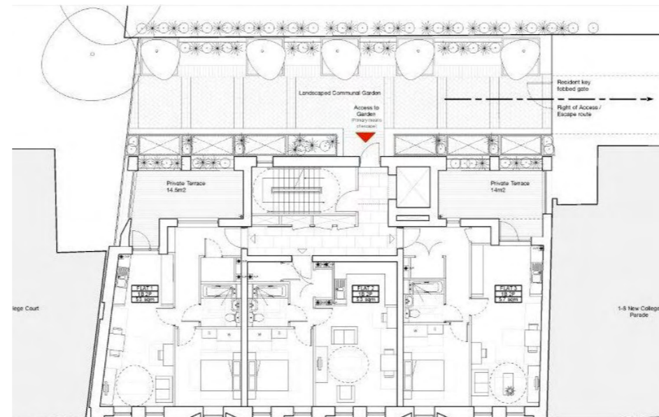
Figure 34: Detail taken from the proposed plan for the first floor level, showing the communal garden at the rear. As shown in this plan, a number of flats will also have a private terrace.
