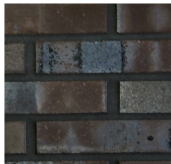
① Textured clinker brick, engobe/ coal fired. Colour - brown/ purple
