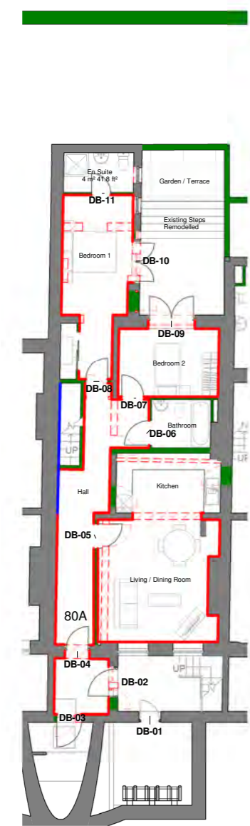
Basement Floor (Skirting details) 1:100
