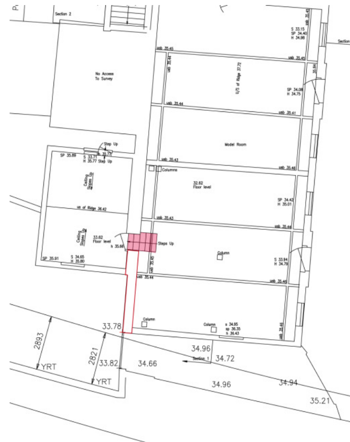
Figure 7: Previous survey of Tack Room upper floor showing west elevation opening in red and wall thickness at the southern end outlined also in red.
