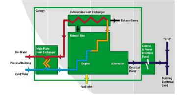
In order to optimize the performance of the CHP engine it is important to provide consistent heating and electrical loads. For this reason, such a system would be supplemented by a gas fired boiler system and public electrical supply.
