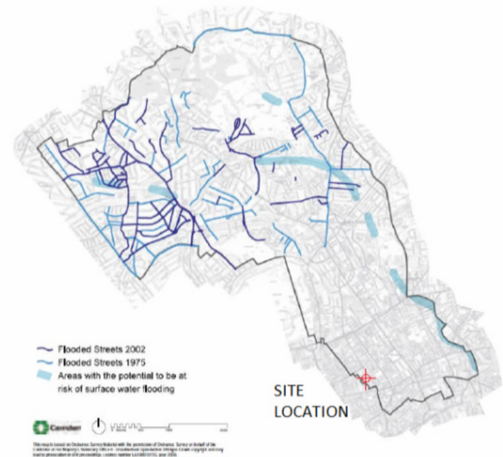
Historic flooding map of Camden (extract from Arup report Camden geological, hydrogeological and hydrological study: Guidance for subterranean development)
