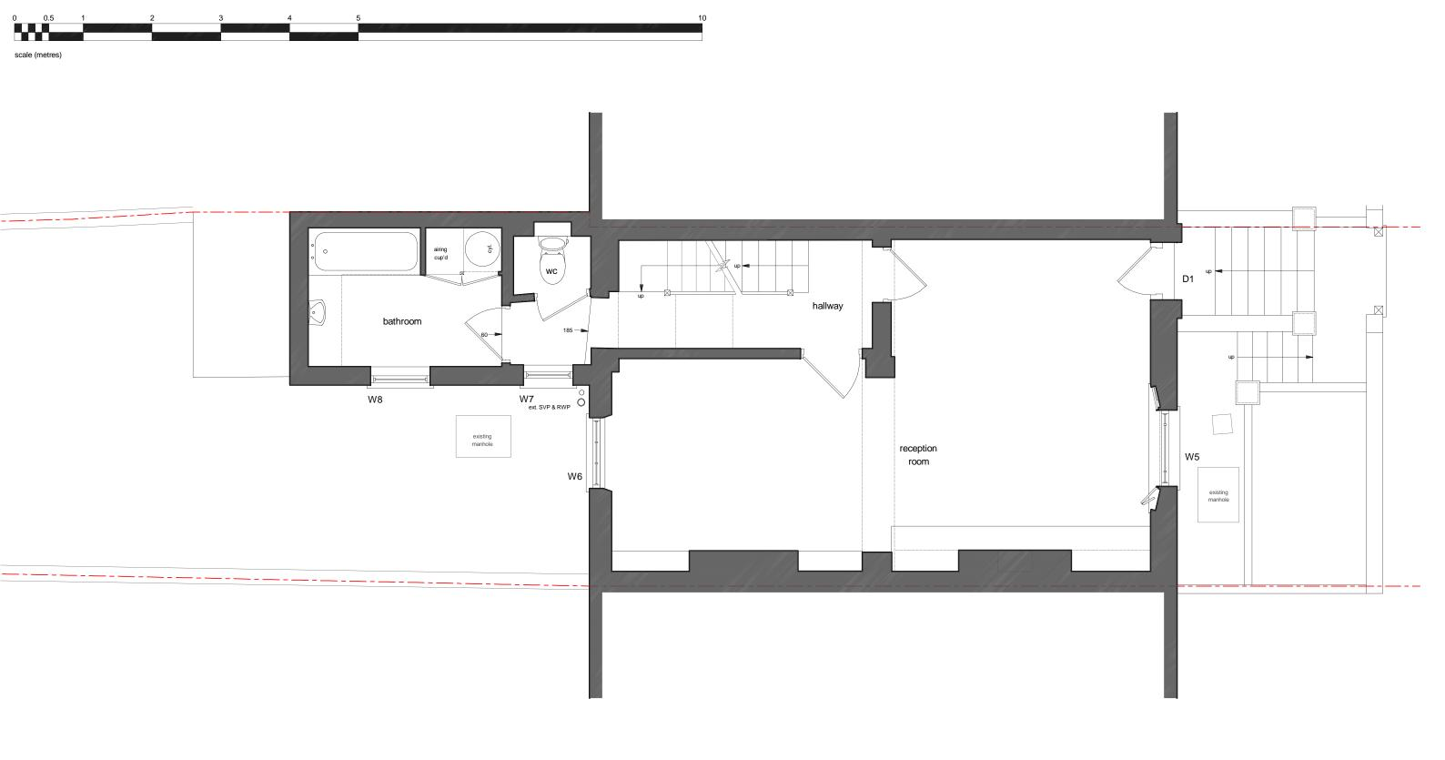
W1, W5, W6, W13 - Repaired W12, W10, W11 - Sash replaced with slim light double glazing in sectional frames
