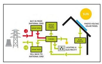
panels that are integrated into a roof are more expensive than those that sit on top. Grid connected systems require very little maintenance, generally limited to ensuring that the panels are kept relatively clean and that shade from trees does not obstruct the sunlight path. However, the wiring and system components should be checked regularly by a qualified technician.
