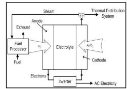
them of their electrons. The hydrogen atoms are now "ionized," and carry a positive electrical charge. The negatively charged electrons provide the current through wires to do work. If alternating current (AC) is needed, the DC output of the fuel cell must be routed through a conversion device called an inverter.
