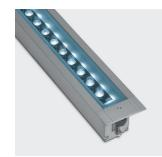
Linealuce Compact recessed - Linear Recessed - 20W 1740Im - Warm White LED - electronic control gear 220-240V ac - L=1658 mm - Wall Washer Optic
