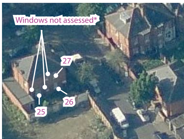
Potentially affected windows on 19 and 19a Richborough Road (*The 3 no. windows that were marked as not assessed are connected to non-habitable rooms, and are therefore not applicable to the BRE Guidelines for daylight and sunlight)
