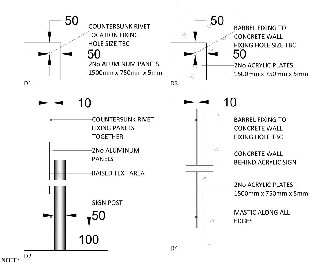
LETTERS WITH STUDS FIXED THROUGH THE FRONT PANEL. THE STUD WOULD BE TACK WELDED TO THE BACK OF THE FRONT PANEL, FILED SMOOTH TO THE SURFACE. THEN THE BACK PANEL WOULD BE FIXED FLUSH TO THE FRONT PANEL.
