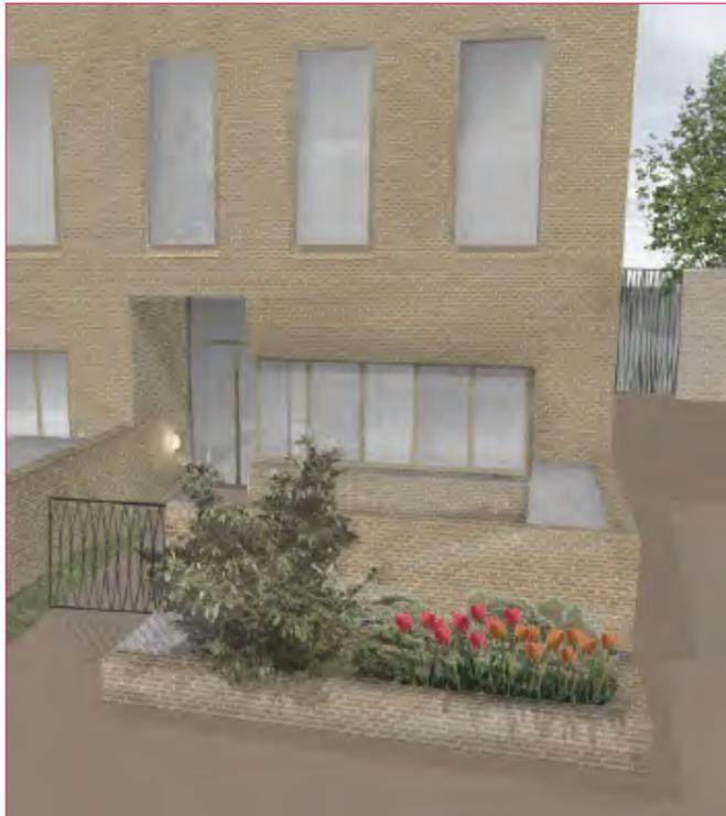
Plot FGHI rear garden walls consist of a low level garden wall with integrated bin and bike storage, 900mm height; a planter of 450mm height defines the boundary.
