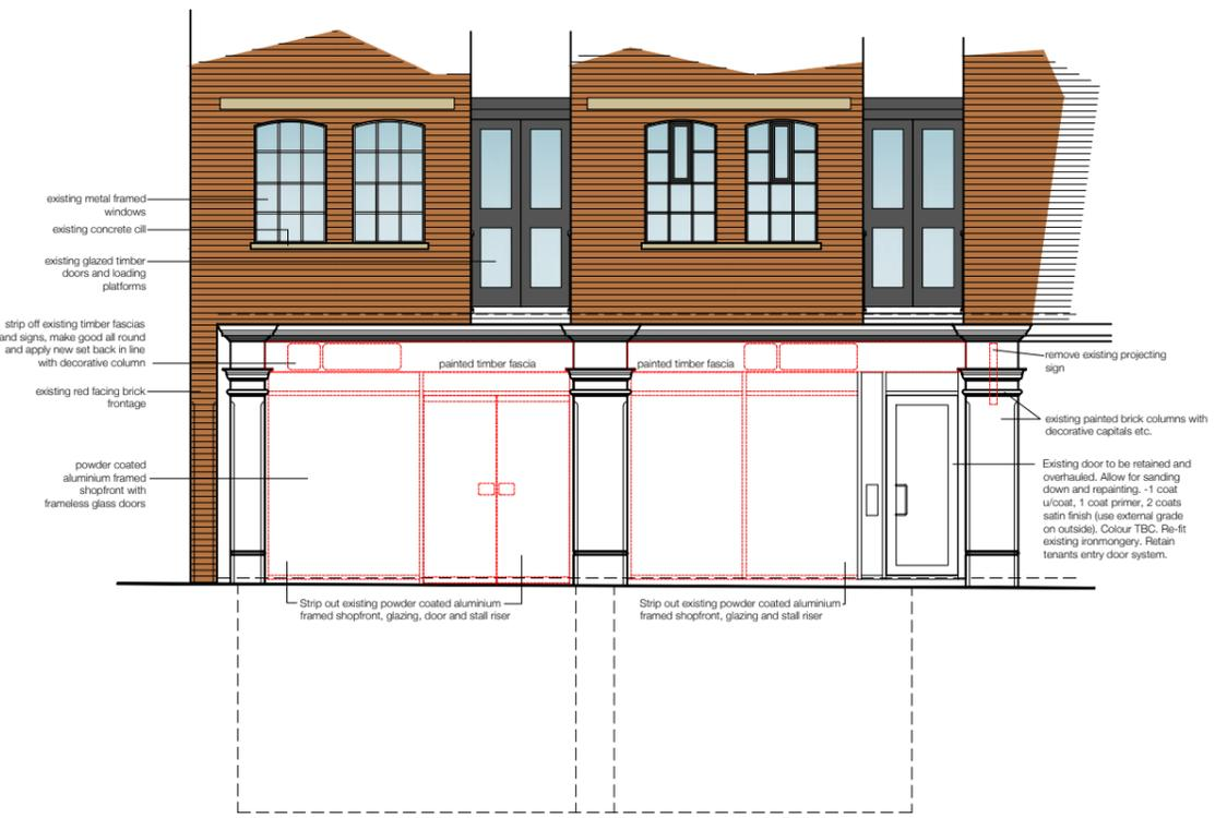
All existing windows being retained. Allow for overhaul of ironmongery, replacement of any broken glass etc. All windows to be thoroughly sanded down and repainted, 1 coat u/coat, 1 coat primer, 2 coats satin finish (use external grade on outside). Colour TBC.
