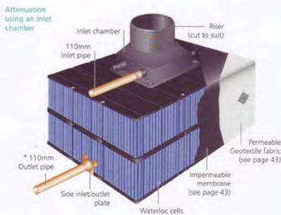
\* Inlet pipes may also be connected to the vertical face of the cell (refer to page 35)
