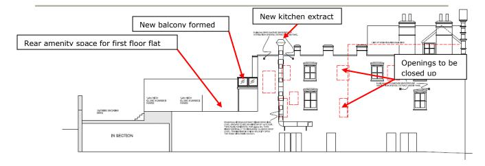
6.9 On the rear elevation existing window openings will be enlarged to floor level so that access can be created onto the roof terraces or balcony. This elevation faces out onto the car park and Stanmore Place beyond. The existing rear elevations of the streetblock comprise a somewhat drab street scene and do not constribute to the character or appearance of the conservation area in a positive way. What is proposed for the application site will have a neutral impact.
