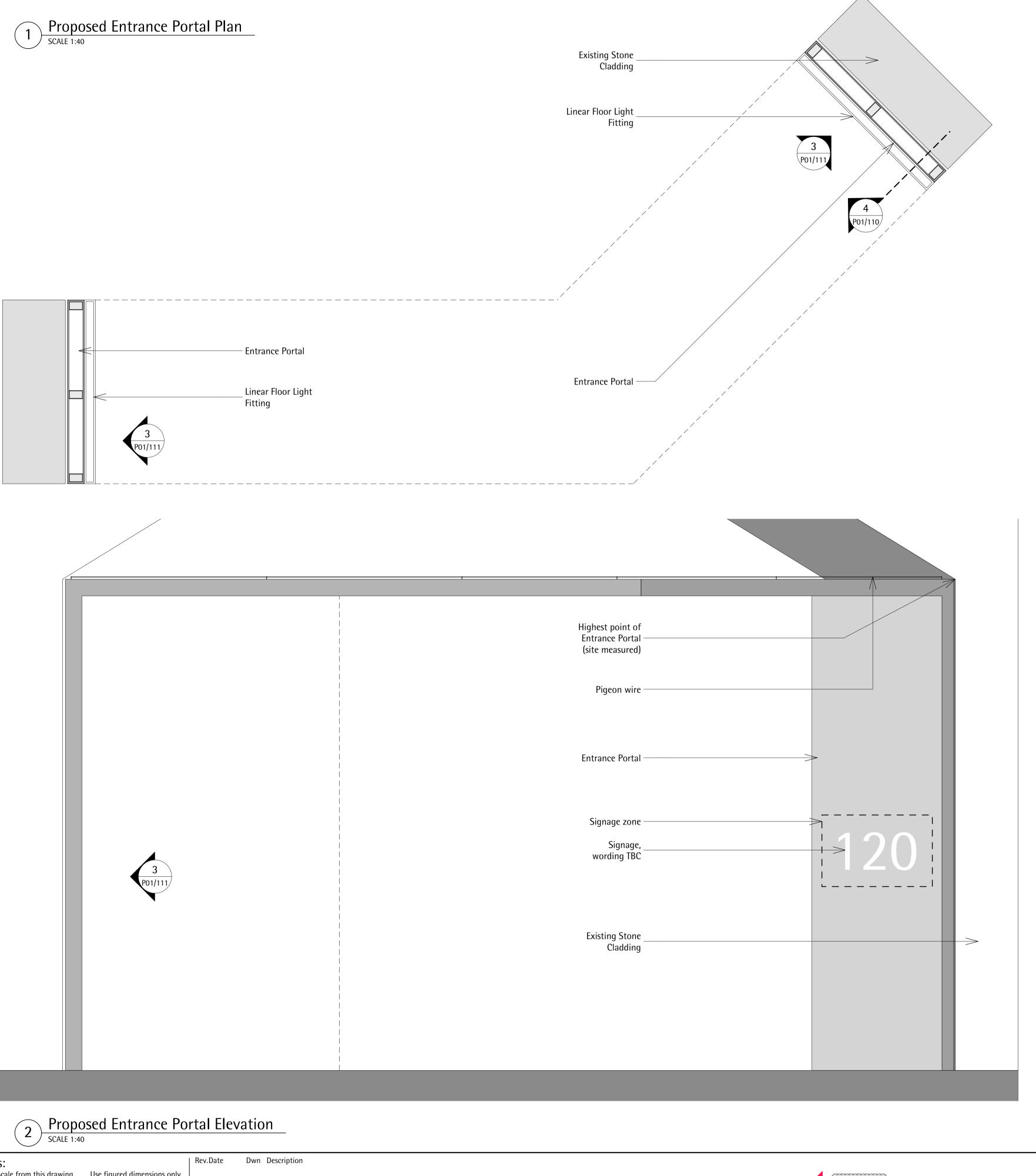
Existing Stone Cladding Linear light \_ fitting Pigeon wire Glazed Entrance Screen Signage zone wording TBC Entrance Portal -
