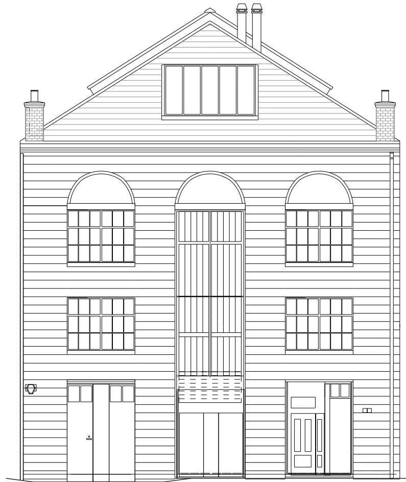
Historic Reconstruction Facade- Based on Archive Photographs Circa 1980
