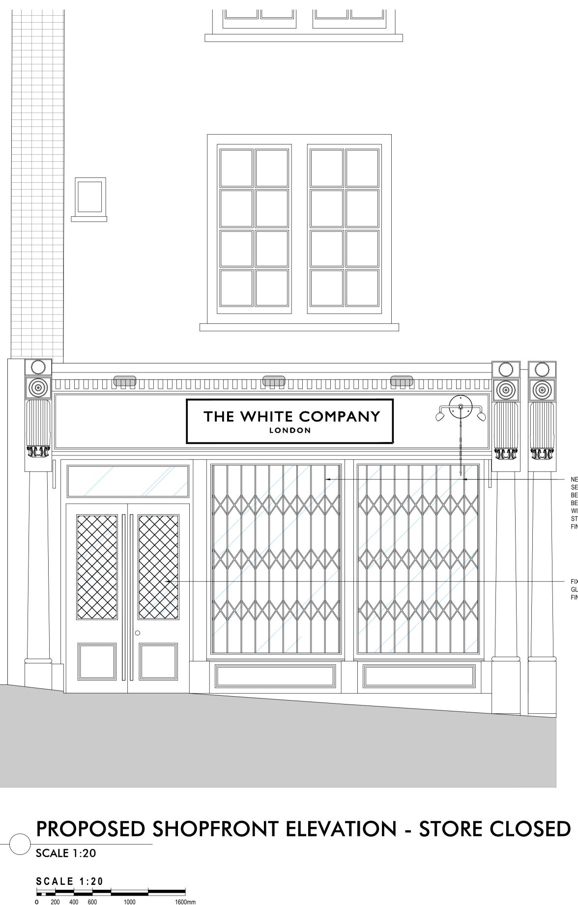
NEW CONCERTINA GRILLES TO BE INSTALLED FOR SECURITY PURPOSES, BEHIND GLASS. GRILLES TO BE OPENED DURING TRADING HOURS. FRAMES TO BE FIXED IN TO NEW FIT-OUT PARTITION. THESE WILL NOT BE FIXED TO THE EXISTING LISTED STRUCTURE. FINISH RAL 9016
