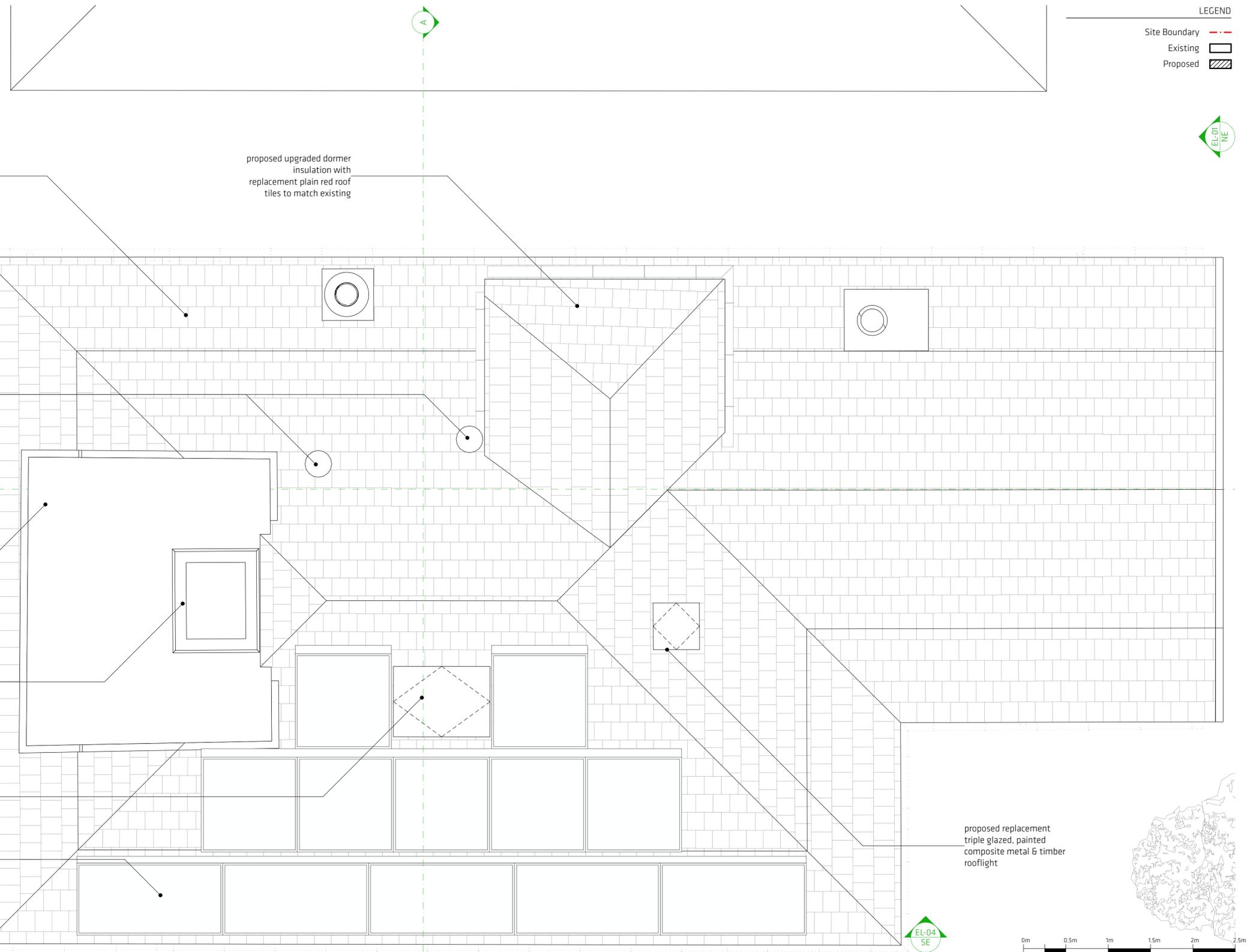
proposed upgraded roof insulation with replacement plain red roof tiles; tiles, roof pitch and geometry to match existing
